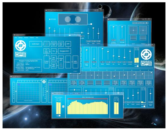
The DPS Profile Creator is a Windows PC application that connects via UART to the SPHE8107 platform. This tool provides comprehensive real-time control over every parameter. Input, output and gain-reduction meters give the audio engineer immediate feedback of the behavior of the algorithm as it is running on the target platform.
